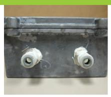
Figure 2. Aluminum housing with ports installed for pressure and temperature probes.
