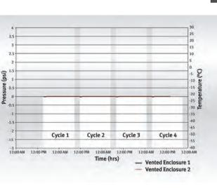
Figure 4. Pressure differentials for vented enclosures.
