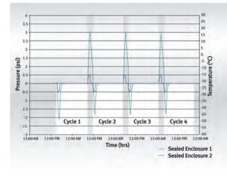
Figure 5. Pressure differentials for sealed enclosures.
