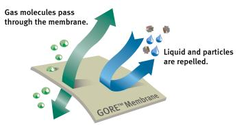
**GORE®** PACKAGING VENTS EQUALIZE PRESSURE, **PREVENTING CONTAINER LEAKAGE OR RUPTURE.**
