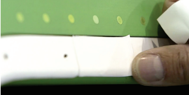
Figure 13: Adhering the replacement tape
