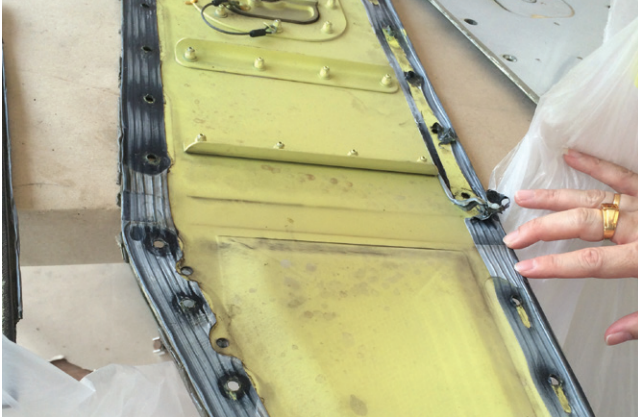
Figure 1: Material torn along edge, torn away from fastener holes, excessively compressed (black), and separating from panel
