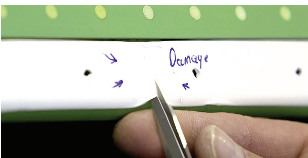
Figure 9: Slitting the damaged section
