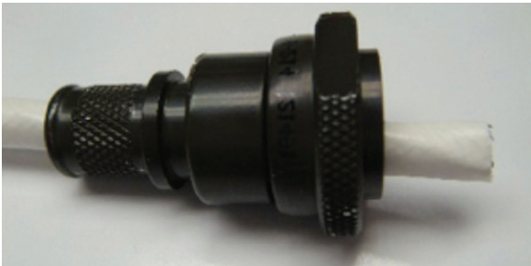
Figure 10: Inserting backshell on the cable
