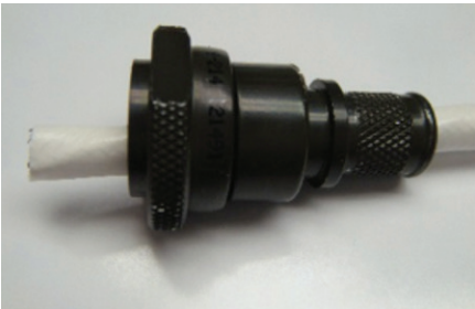
Figure 42: Inserting backshell on the cable
