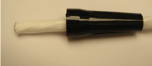
Figure 8: Attaching the connector cap
