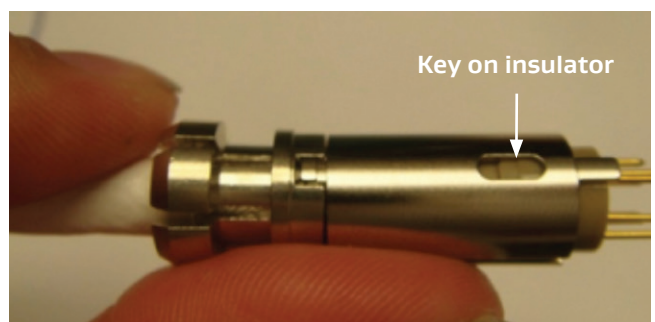
Figure 43: Insulator key for alignment
