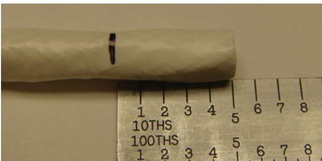
Figure 10: Marking the cable
