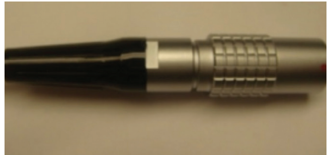
Figure 45: Installing the connector cap on socket end
