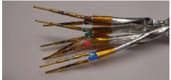
Figure 17: Stripping the pairs
