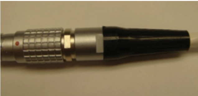
Figure 44: Installing the connector cap on plug end
