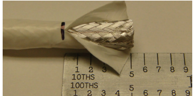
Figure 29: Slitting the cable jacket
