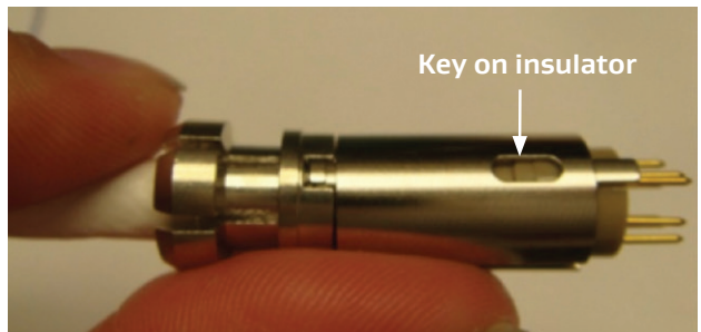
Figure 25: Insulator key for alignment
