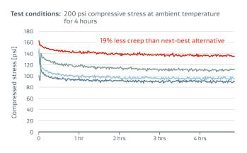
Gore's creep resistance means fewer adjustments and less water wasted.
